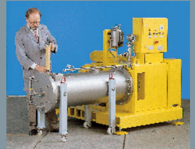
Fig. 7.1: PMC SuperTex® 140 – Removal of a ceramic modular separator
