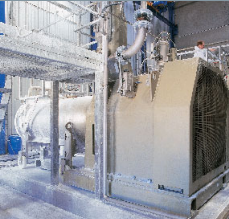
Fig. 6.1: SuperTex® 1200 in wet grinding plant for white pigments
