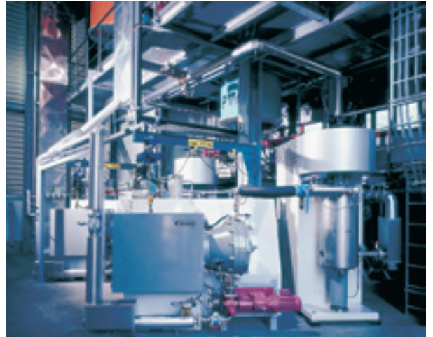
Fully automatic offset line. Throughput 1000 kg/h.
